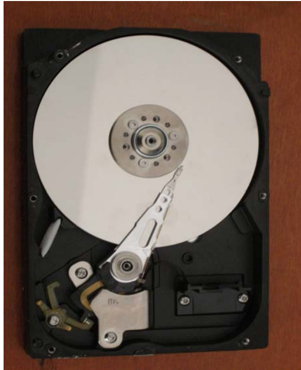
Fig1. Disk drive head control system
