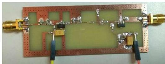
Fig. 5 Photograph of cascaded power amplifier
