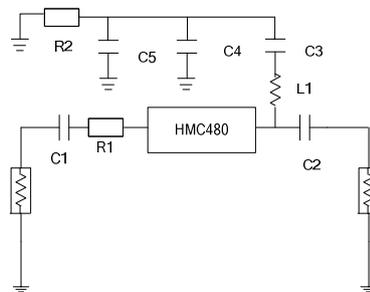
Fig. 1 Circuit schematic of driver stage power amplifier.
