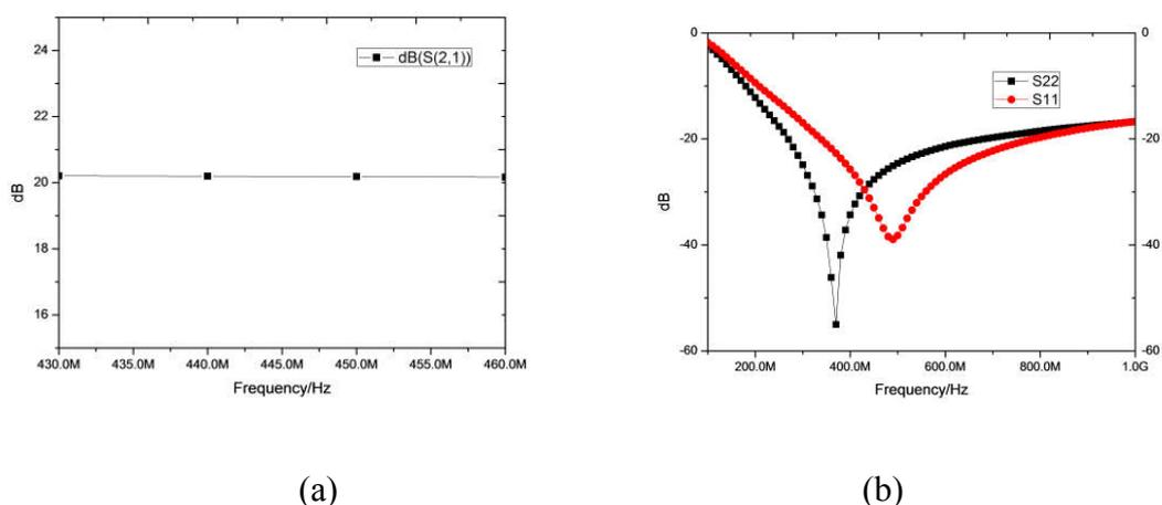
Fig. 2 The S parameters simulation of the drive stage power amplifier.
