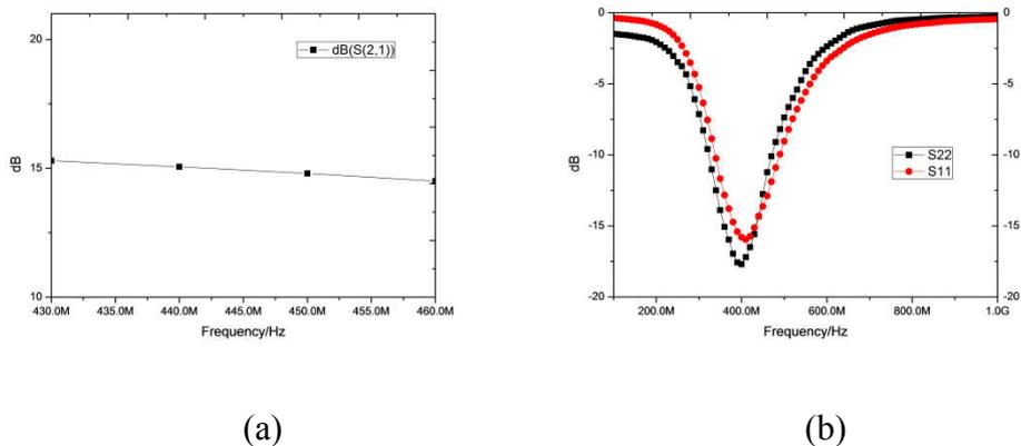
Fig. 4 The S parameters simulation of the final stage power amplifier.
