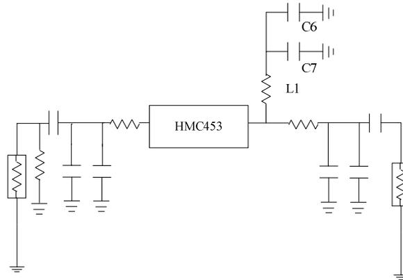
Fig. 3 Circuit schematic of final stage power amplifier.
