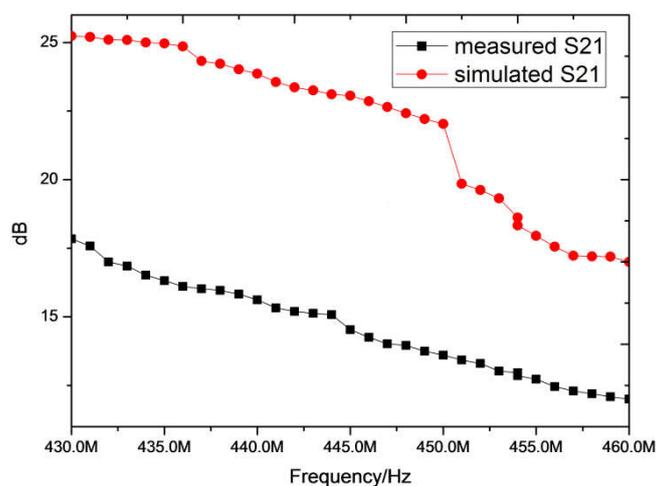
Fig. 6 Simulated and Measured S21 of the cascaded power amplifier
