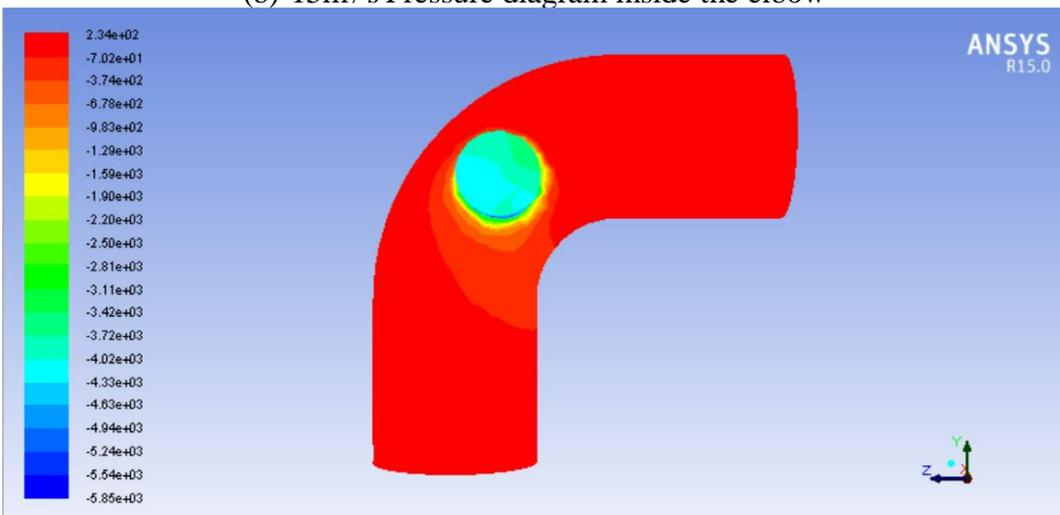
(c) 20m/s Pressure diagram inside the elbow
