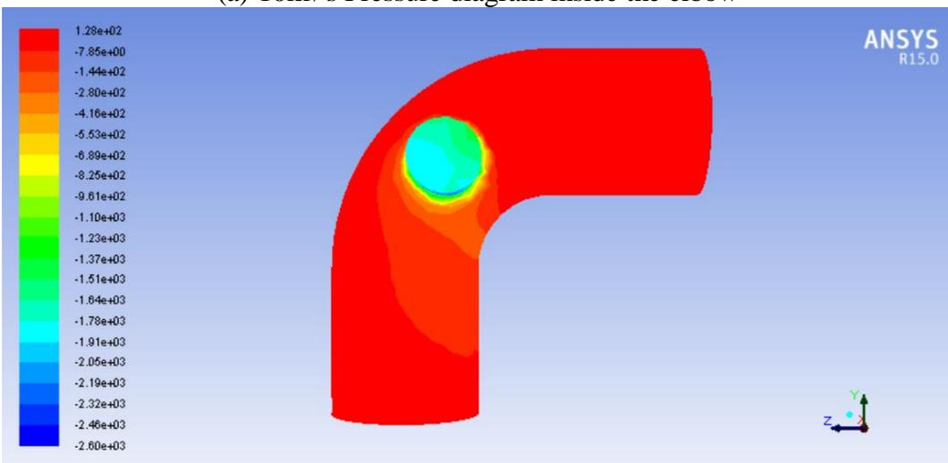
(b) 15m/s Pressure diagram inside the elbow
