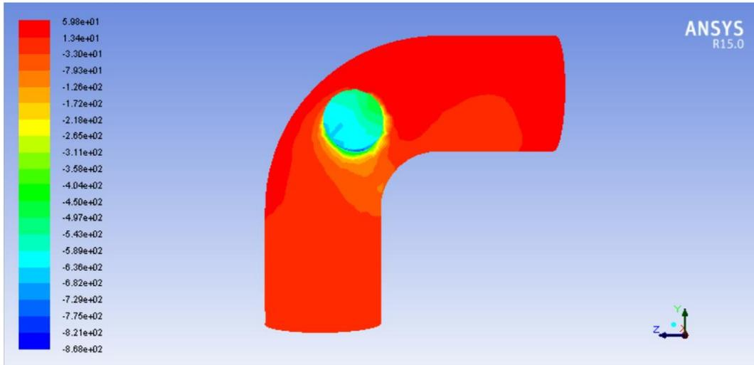
(a) 10m/s Pressure diagram inside the elbow
