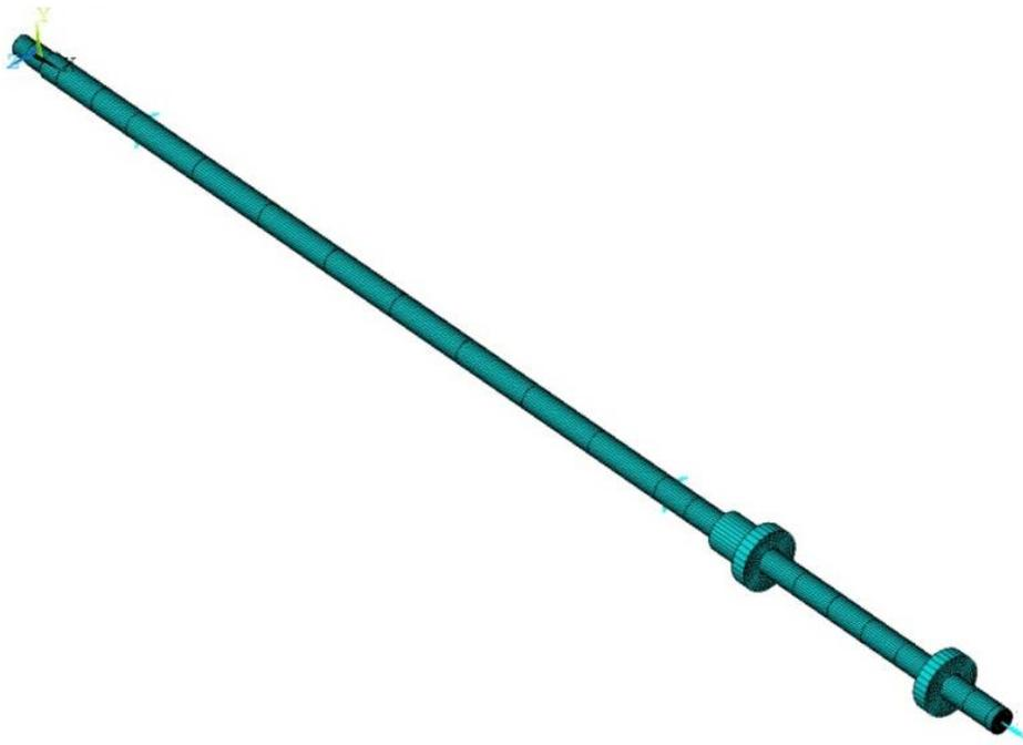
Fig.2 Finite element model of the marine propulsion shafting
