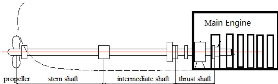
Fig. 1 The diagrammatic sketch of the marine propulsion system
