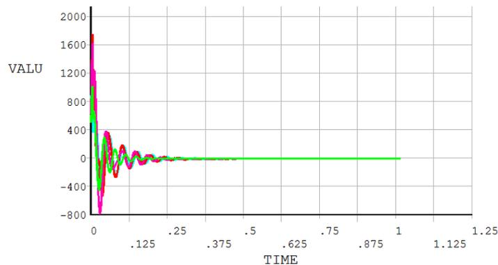
Fig. 4 The attenuation curve of the bearing reaction force under the impact load
