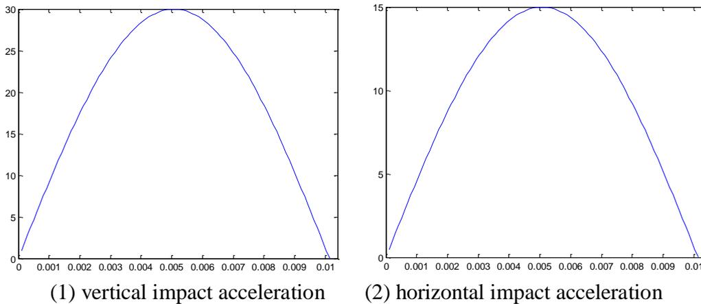
Fig. 3 The acceleration shock wave and time history curve of the propulsion shafting
