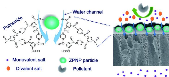
Figure 11. Schematic illustration of the microstructure and separation performance of the TFN-ZPNP membrane. Image reproduced from Yan-Li Ji et al. [33]
