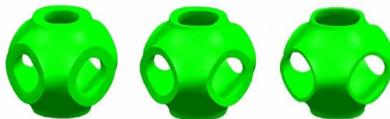
Fig 2. P structure with 70%, 80% and 90% porosity
