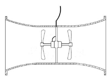
Figure 1. Sectional view of water flow generator
