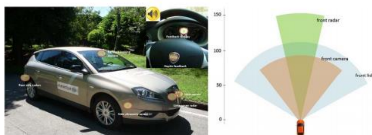
Fig 2. Left: Examples of AVs. Right: Field of view of the three frontal sensors (Chavez, 2016)
