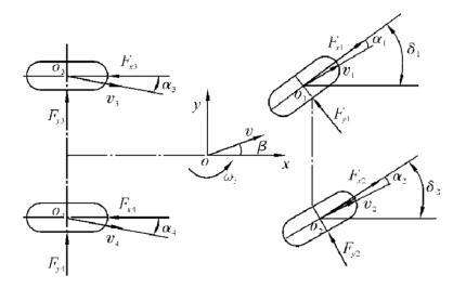
Fig 1. Vehicle dynamics model
