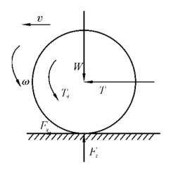
Fig 2. Force analysis of driving wheel
