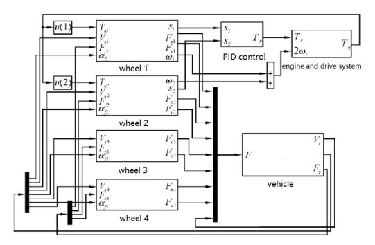
Fig 3. EDS control system model
