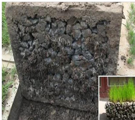
Figure 8. Ecological porous concrete greening method
