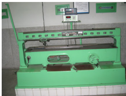
Fig 9. Lcc-1500 chain length measuring instrument
