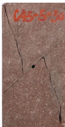
(a) Red sandstone loading failure mode diagram (b) Unloading failure mode diagram of red sandstone
