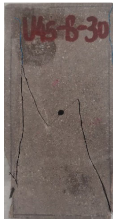
(a) Red sandstone loading failure mode diagram (b) Unloading failure mode diagram of red sandstone
