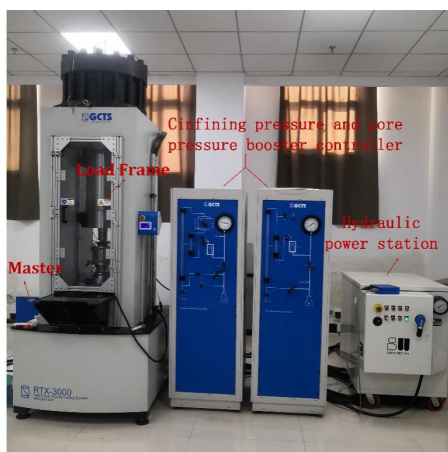
Figure 2. GCTS RTX-3000 rock mechanics system
