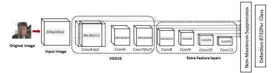
Figure 1. SSD Network Structure Diagram
