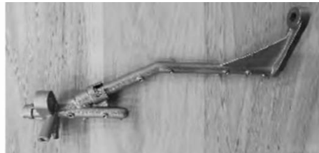
Figure 5. Transmission drencher assembly
