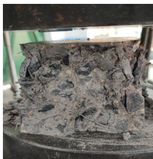
Figure 1. Compression failure pattern of steel fiber reinforced recycled concrete
