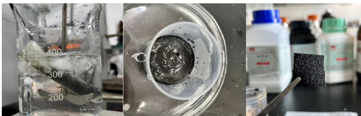
Figure 2. Preparation of PANI/PPy/CC hydrogel electrode
